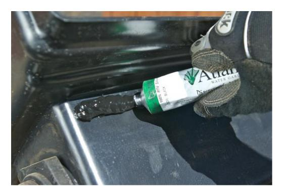
Using the included silicone sealant run a continuous bead across the circle of screw holes on the back of the spillway.
