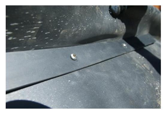
Once all screws have been inserted and tightened carefully trim away the liner inside the compression fitting.
